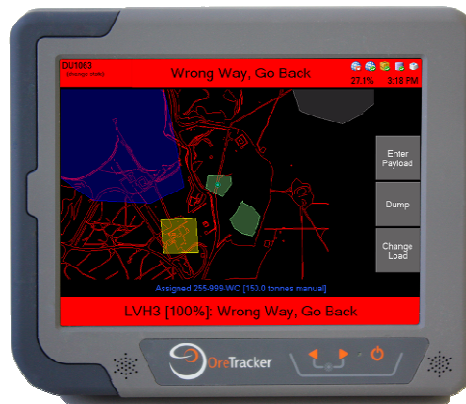
Figure 4 –OreTracker console showing driver warning display
